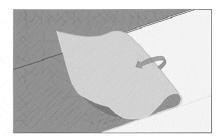
**4.4.** Never pre-cut material to final trim until it is placed into the adhesive. Leave material 2"-3" longer for trimming after placement.
